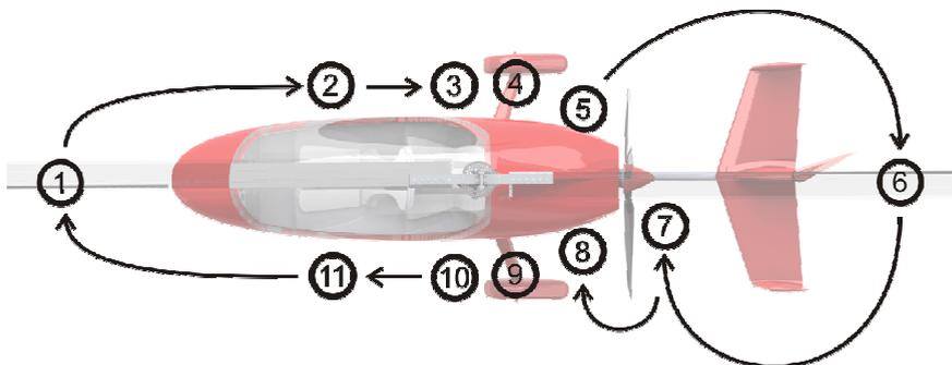
The following checks must be carried out before each flight. However, if the gyroplane is operated by a single pilot or within an organization where the checks are performed by or under the supervision of qualified personnel, check list items marked with a preceding 'O' may be carried out daily, before the first flight of the day.
