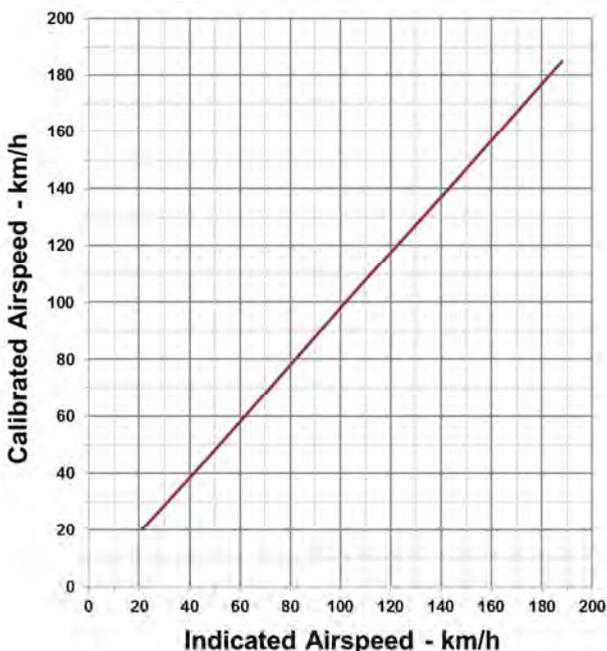
**Example:** Indicated airspeed of 140 km/h represents a calibrated airspeed (corrected for installation error) of 138 km/h.
